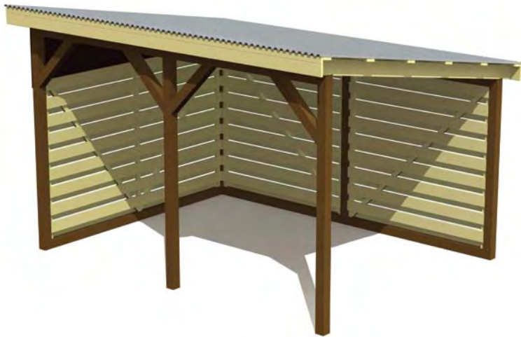
VP001 Shelter with wooden floor, 3x4m (two walls and plastic roof)
